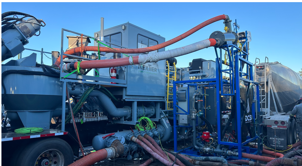
The 7' x 7' DriFlow X unit gravity feeds hydrated product direct to the blender tub.
