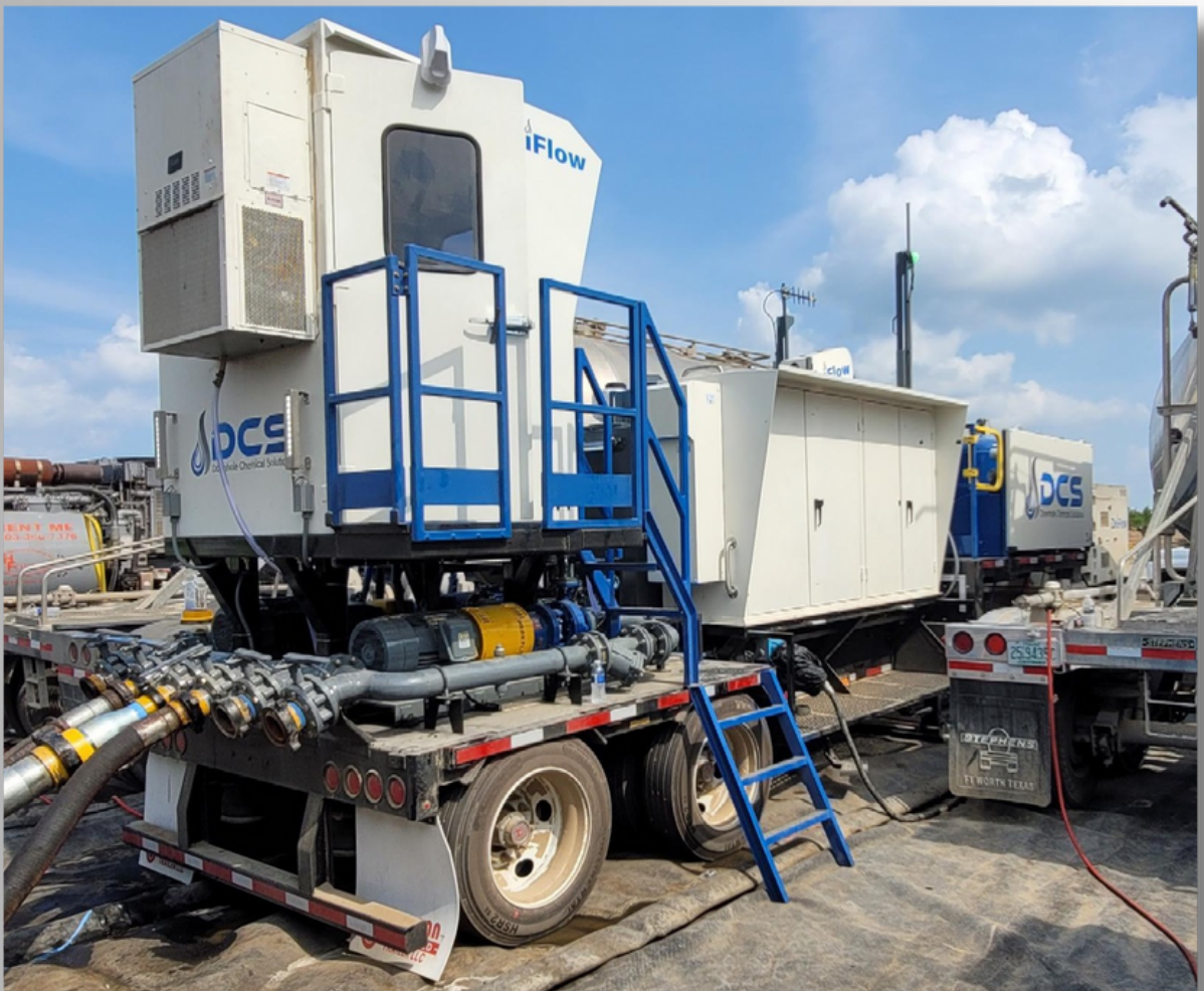
DriFlow Unit 3.4 pumping guar in the Haynesville basin.
